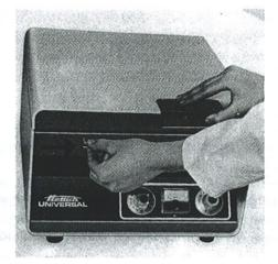
3.1.8 Opening of thelid inthe event of power failure or breakdown.Insert the wire rode (included in the accessories) up to its half length, into the hole. On swinging it clockwise, the tumbler
