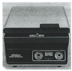
3.1.7 After lapse of the set time, the lid-locking disengages. Then the lid can be opened.
