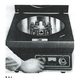
Set the time switch to the required centrifugation time, For required times less than 5 min,the switch must first be set to approx.15-20 min and then set to the required time. If the time switch is not switched on the lid cannot be closed. At the end of the period the centrifuge switches off automatically and is then rapidly and gently brought to a standstill with a 2-stage brake.
