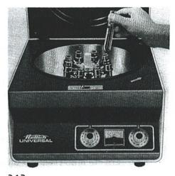
3.1.3 Take care in so doing that the rotor is well balanced. Pay attention that the same quantity and size of suspensions, tubes and rubber inserts are always used in opposite.
