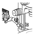
The thread connector also enables the lampholder to be connected to the cast foot.
