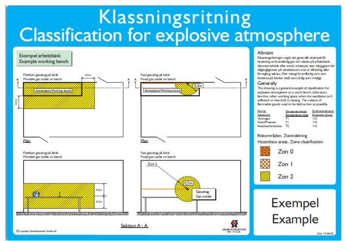
In general zone 2 applies within a distance of 0.5 m on the side above and below the bench surface when handling free gas bottles. At a fixed outlet, zone 2 applies within a radius of 0.5 m around the outlet.
