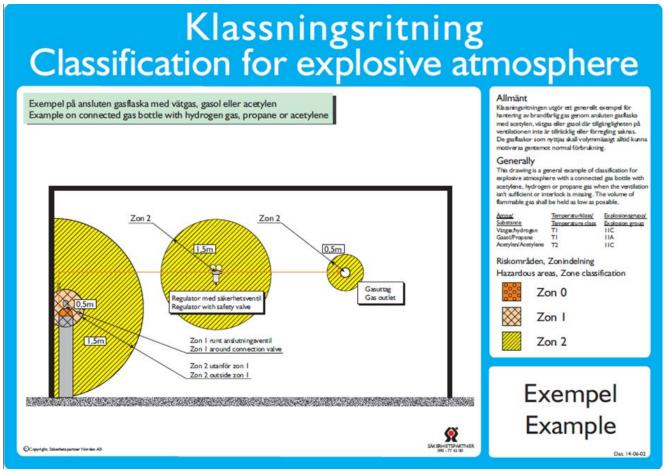
Zone 1 applies with a radius of 0.5 m around the connection valve and Zone 2 in a radius of 1.5 m outside Zone 1. Around a regulator with safety valve for Zone 2 applies with a radius of 1.5 m. For outlets Zone 2 applies within a sphere with a radius of 0.5 m around the outlet mouth.
