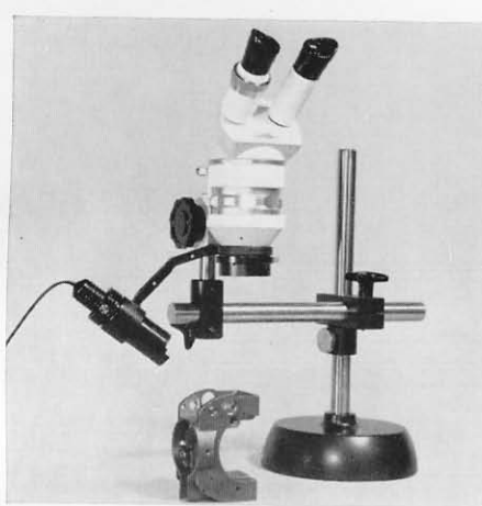
Fig. 5 M5 stereomicroscope with 0.5 × additional objective on swinging arm stand
